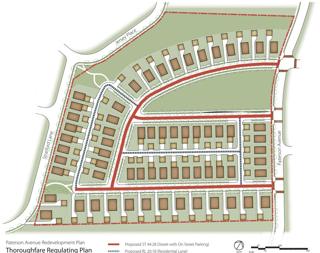
The thoroughfares serving the proposed Area have a recommended range of lanes, turning movements, and parking arrangements. The specific design and geometries of the improvements should be determined by the Town's Engineer. Each typology is illustrated and codified in the Thoroughfare Sections.
